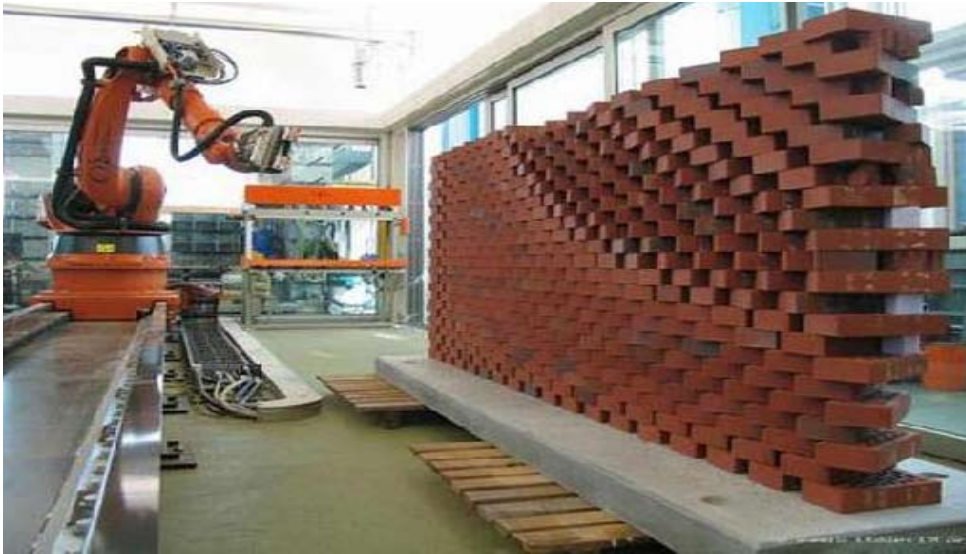
Figure 11. Construction de murs robotisée, Gramazio Koler Architects (source : www.electronicsoffline.com ).
